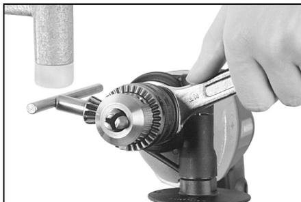
Hold the drill spindle tight with a spanner. With a light blow from a rubber hammer, release the chuck from the inserted chuck key and unscrew it.
