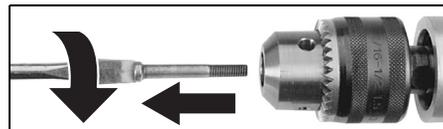
Undo the locking screw. THIS SCREW HAS A LEFT-HANDED THREAD!
